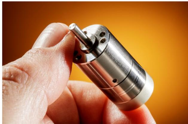
The motor construction is based around the established friction drive method which results in good self-locking characteristics meaning that the motor can hold position without consuming any power. The integrated 15 bit magnetic absolute encoder gives a closed loop resolution of 0.2 milli-radians (0.01°), and as always with the Piezo LEGS technology, you get an amazing sub-micro-radian resolution in open loop.
