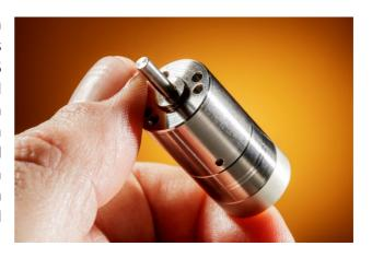
The motor construction is based around the established friction drive method which results in good self-locking characteristics meaning that the motor can hold position without consuming any power. The integrated 15 bit magnetic absolute encoder gives a closed loop resolution of 0.2 milli-radians  $(0.01^{\circ})$ , and as always with the Piezo LEGS technology, you get an amazing sub-micro-radian resolution in open loop.
